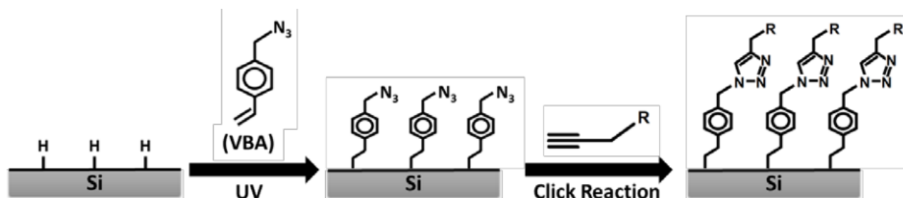
Figure 1. A hydrogen-terminated silicon surface is transformed to an azide-terminated surface using an organic azide (ex. VBA) and UV light (step 1). The modified surface can then undergo a click reaction to attach probe molecules such as for biosensing applications (step 2).
