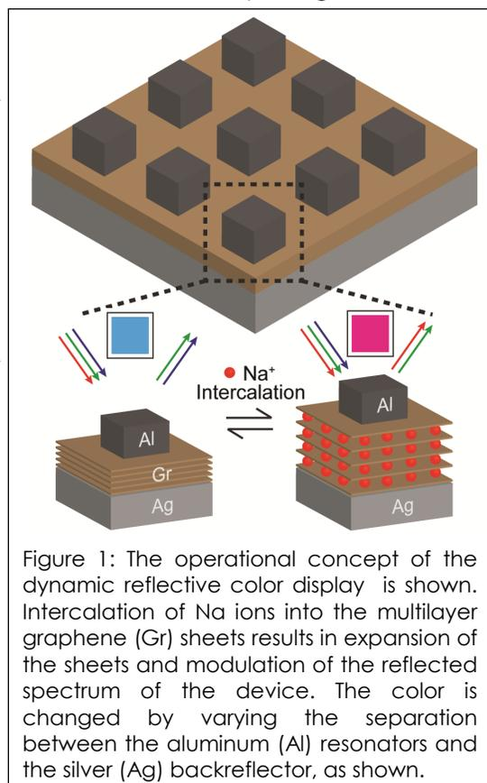
Figure 1: The operational concept of the dynamic reflective color display is shown. Intercalation of Na ions into the multilayer graphene (Gr) sheets results in expansion of the sheets and modulation of the reflected spectrum of the device. The color is changed by varying the separation between the aluminum (Al) resonators and the silver (Ag) backreflector, as shown.
